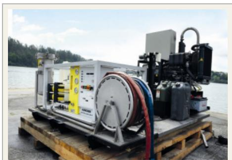
The WPU can clean up to 500 litres of water per hour for construction and drinking.
