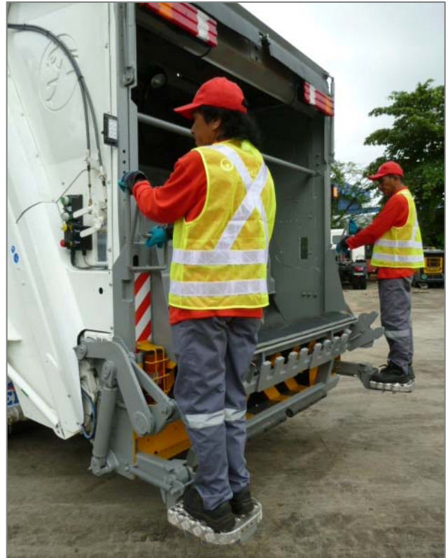
Large-sized foldable rear-platform interlock with speed and reversing.
