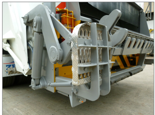
Large-sized foldable rear-platform interlock with speed and reversing.
