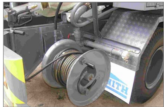
Rear mounted hose-reel with hand-lance for general hi-pressure washing .
