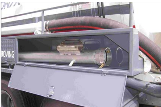
Hose compartment on both sides of tank for 150mm dia hose of 3m lengths.
