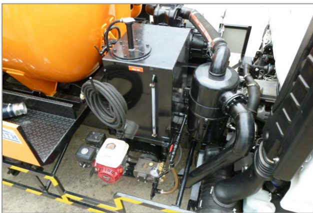
Designed to ASME Sect VIII 2 bar working pressure
