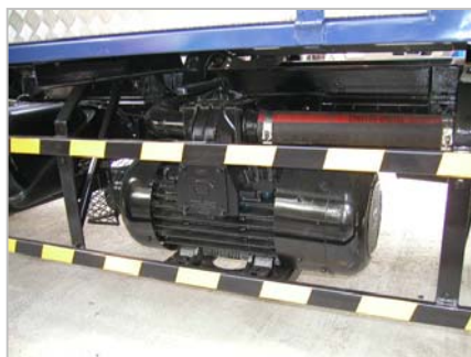
Air-cooled Moro Vacuum Pump, model AC5 with Free-Air Flow 780m 3 /hr (459cfm) Max vacuum = 95% Max Press = 1 bar Power req'd for max vacuum = 19 kW
