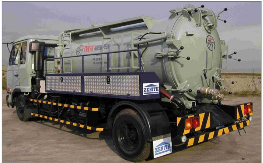
Model VCT-50 Design Code = ASME Section VIII for sludge waste 5,000 ltr Vacuum Tanker on Nissan chassis 4 x 2 10.5 MT GVW chassis . Shell thickness typically 6.0mm (upto 8.0 mm upon request) of ABS grade A ship plate , internally coated with coal tar epoxy. Tipping Cylinder and hydraulically operated rear-door for easy maintenance and cleaning operation.
