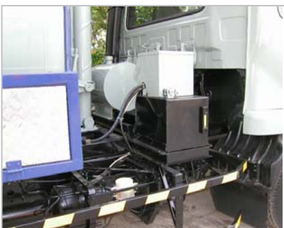
DC-power operated hydraulic power pack for tipping and rear-door.
