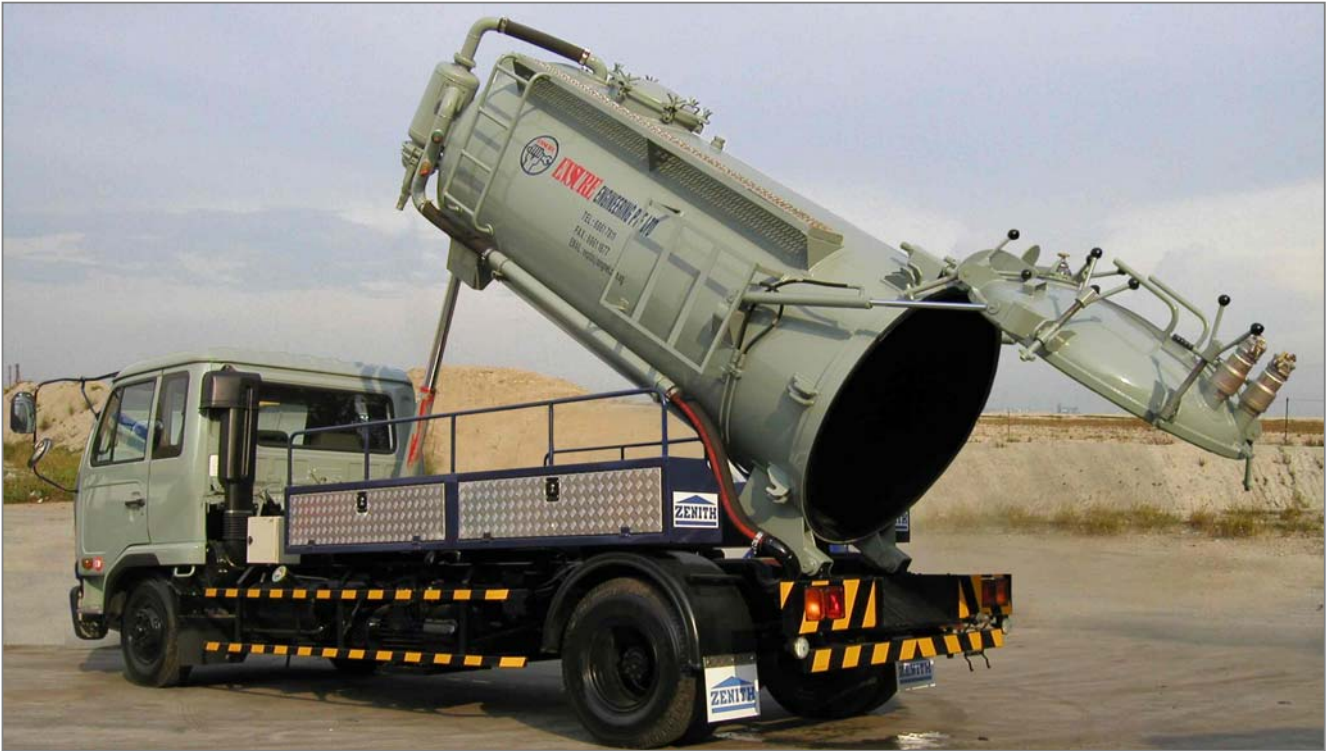
Model VCT-50 Design Code = ASME Section VIII for sludge waste 5,000 ltr Vacuum Tanker on Nissan chassis 4 x 2 10.5 MT GVW chassis . Shell thickness typically 6.0mm (upto 8.0 mm upon request) of ABS grade A ship plate , internally coated with coal tar epoxy. Tipping Cylinder and hydraulically operated rear-door for easy maintenance and cleaning operation.
