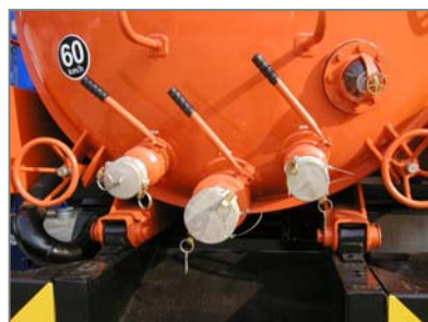
2 x 3" suction and 1 x 4" discharge ball v/v
