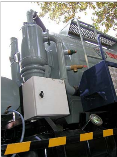
Model VCT-50 Design Code = ASME Section VIII for sludge waste 5,000 ltr Vacuum Tanker on Nissan chassis 4 x 2 10.5 MT GVW chassis . Shell thickness typically 6.0mm (upto 8.0 mm upon request) of ABS grade A ship plate , internally coated with coal tar epoxy. Tipping Cylinder and hydraulically operated rear-door for easy maintenance and cleaning operation.
