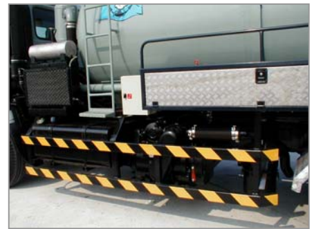
Vacuum Pump-model PR150 with Free-Air Flow of 150 lpm (530 cfm) . Max pressure 2 bar .
