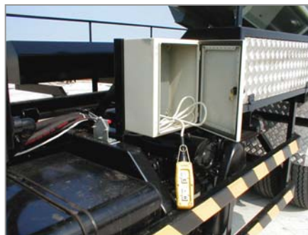
Remote control for tipping operation & remote throttle lever
