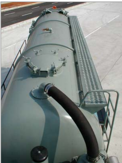
Anti-slip catwalk , manhole, primary and secondary shut-offs. Pressure and vacuum relief valves
