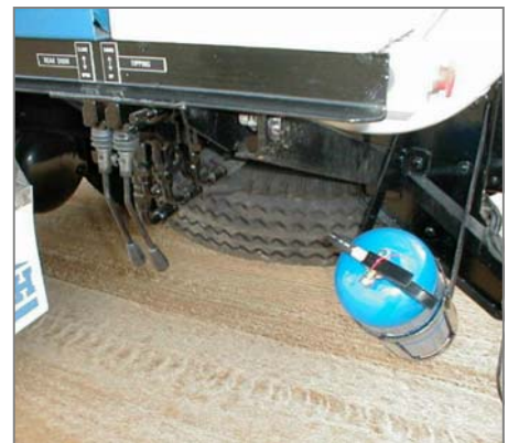
Hydraulic control levers for tipping and rear-door opening.
