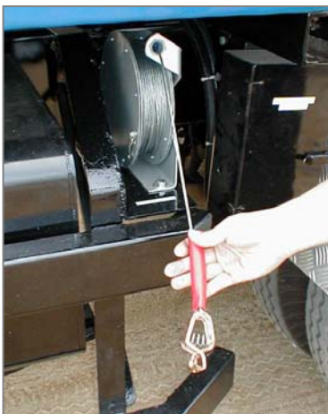
Earthing Strap (mandatory for refinery operation)
