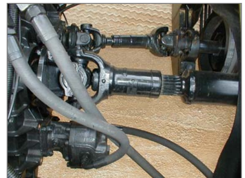
Driven by Split-shaft PTO a) vacuum pump via pulley b) hydraulic pump via direct drive
