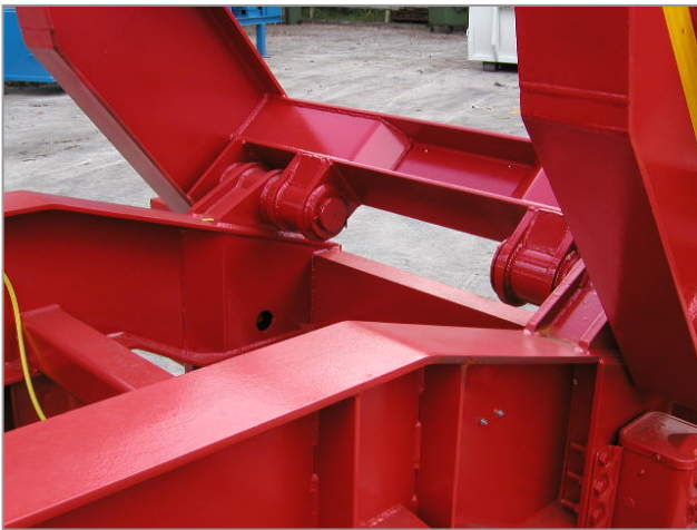
Chassis frame : High-tensile steel 18" x 6" I-beam with re-inforced cross member. Tipping frame : 16" x 7" I-beam c/w suitable cross-member for container twistlocks
