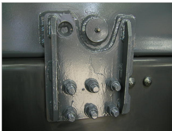
Suitable off-road mounting brackets complying to European truck-manufacturer's recommendations.
