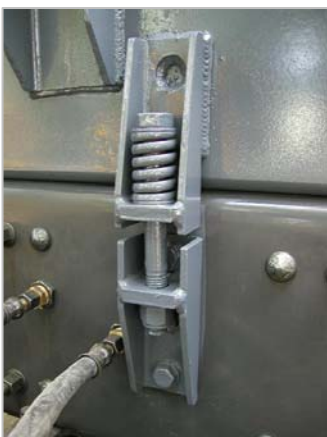
Suitable off-road mounting brackets complying to European truck-manufacturer's recommendations.
