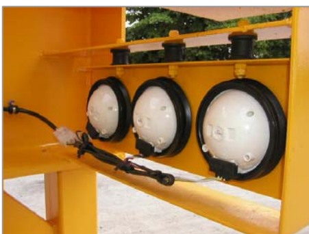
Rear-Light cluster for ease of maintenance & replacement
