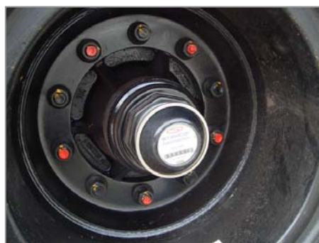
Hubometer to record the distance traveled
