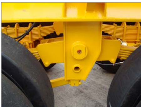
Axle Equalizer for better load distribution
