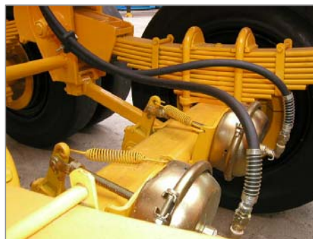
Single Diaphragm Brake Chamber for 1 st & 2 nd Axles
