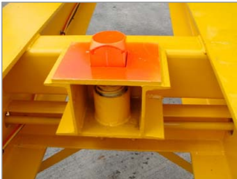
Auto Stopper pin for single container carriage
