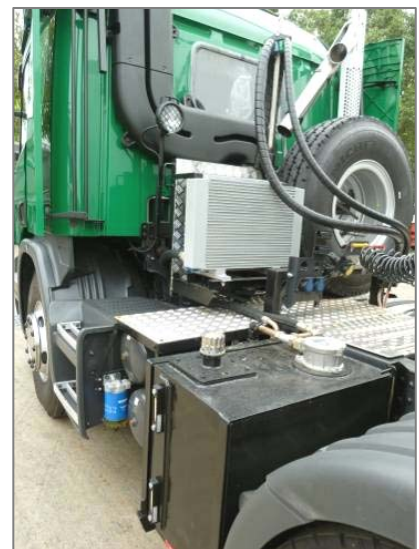
Hydraulic Tank & cooling system
