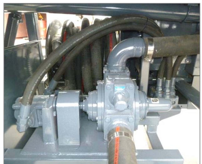
3" diameter hydraulically-driven discharge pump (approx 980 l/min @ 640 rpm)
