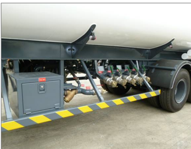
Discharge outlets on both sides of tanker
