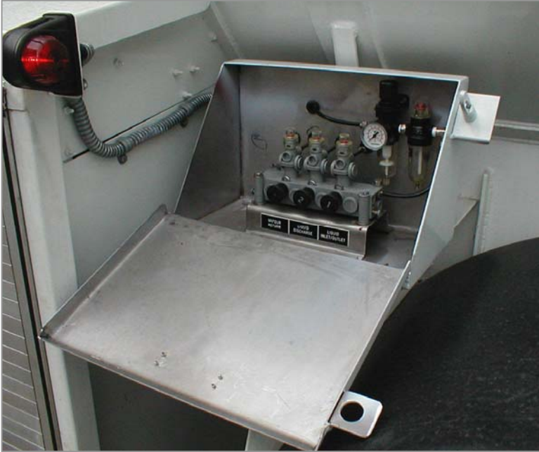
Full Pneumatic control and Emergency shut-off switch.
