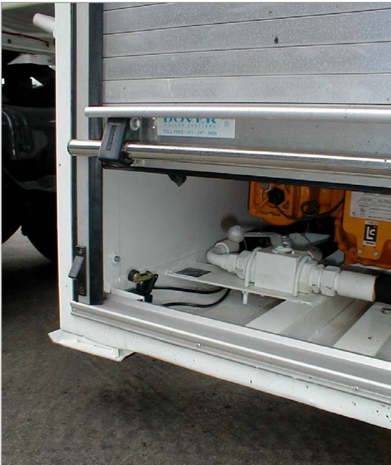
High quality cabinet with spring-loaded positive-lock (ie door will not dis-lodge on rough roads) aluminium Roller-shutter door, pneumatically interlocked to the vehicle brake system.
