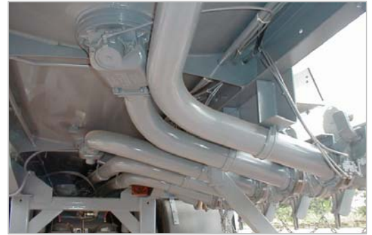
Full-length pipes without weld reduces risk of cracks. (note : Shell Msia prefers API outlet to be horizontal for easy coupling to loading arm)
