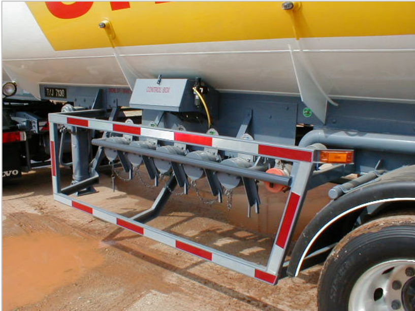
Side-guard made of rectangular box-section for rigidity or option for light weight "C" channel . Side-guard and lock-gate for API cap, API lever, Vapour recovery and electrical socket.
