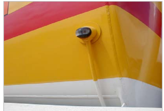
LED side lights and aluminium conduit for durability .
