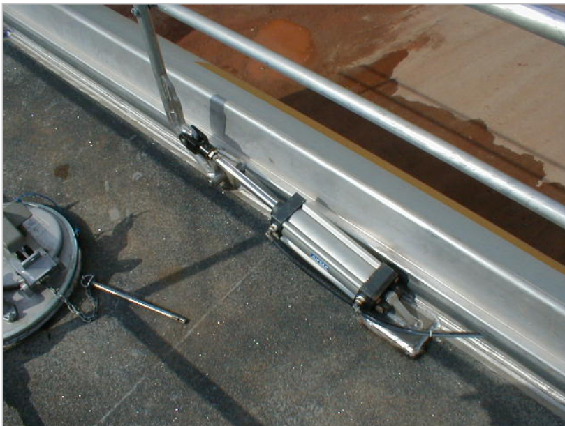
Auto Pneumatic-operated handrail interlock with the trailer brakes , meaning vehicle cannot move when handrail is still up.
