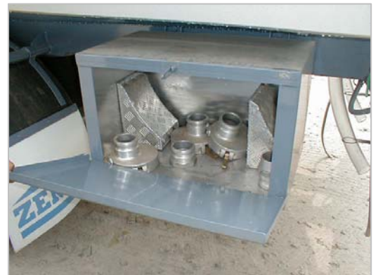
Aluminium alloy tool box on 1 or both sides for adaptors or traffic-cones.
