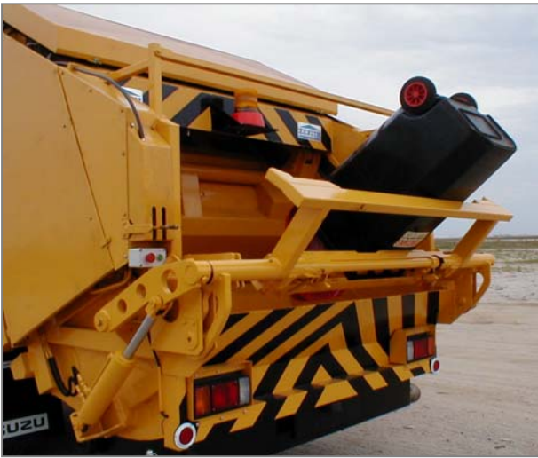
Pictured above is the standard design of Zenith Binlifter for use in Singapore with trunion-arm suitable for HDB metal bins and is also compatible with the HDB CRC dustscrew collection.
